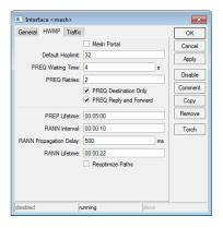
Mesh portal - whether the interface is a portal in the mesh network, if it's set to yes protocol use tree based topology
