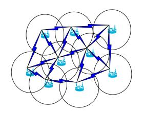
The most common type of configuration: 2.4GHz access points for client connectivity and 5GHz for mesh interconnection.
